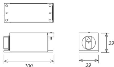
The laser head is available with shutter for stand alone application and without shutter as OEM version.
